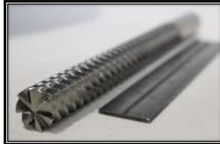
1-1/4" DIAMETER X 8" LOC X 12" OAL 55 DEGREE HELIX
