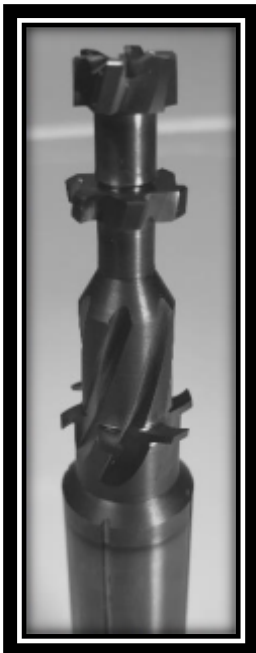
HYDRAULIC VALVE MANUFACTURER. MULTIPLE GROOVES EXECUTED WITH ONE TOOL. THREE OPERATIONS REDUCED TO ONE.
