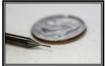
MICRO TOOL DIVISION DRILLS AND END MILLS DOWN TO .003 DIAMETER
